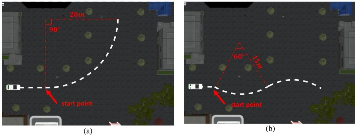
**Figure 6.** Test Scenarios: (a) a 90-degree bend with radius of curvature equal to 20m; (b) a S-Curve with radius of curvature equal to 15m. The white dash line is the designed track.
