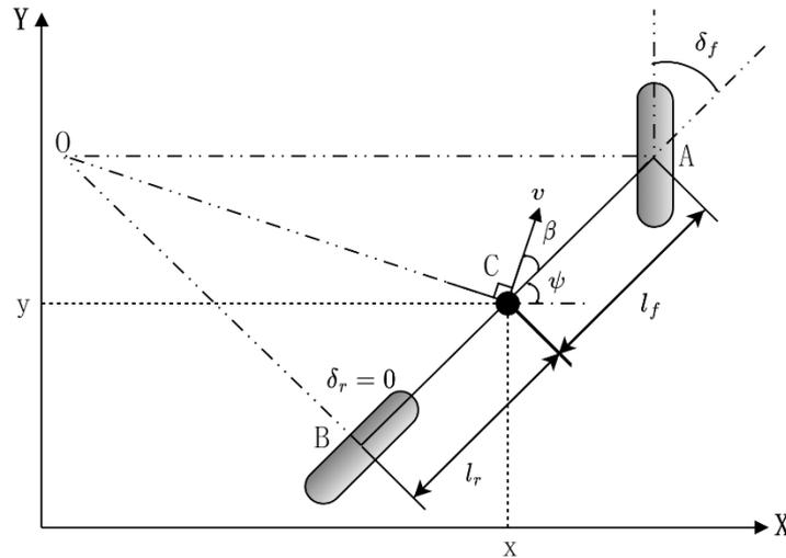
**Figure 2.** *The Two-Wheel Kinematic Bicycle Model.*
