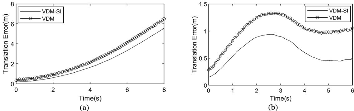
**Figure 7.** *The Translation Error of VDM and VDM-SI Based Navigation: (a) along the 90-degree bend; (b) along the S-Curve. Note that Time = 0s means that the vehicle just entered the start point of the bend of the S-Curve.*
